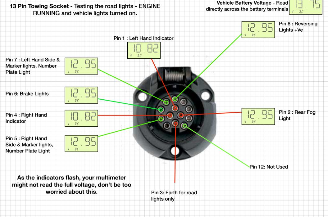
File: 13 Pin Towing Socket-Fault Finding 04
