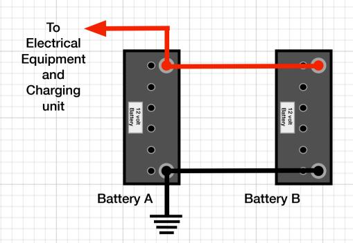
The WRONG way to connect two batteries in parallel.
